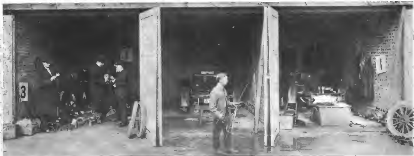
Committee of the Royal Automobile Club Mixing the Parts of the Three Cadillacs, and Handing Out Set for No. 1 Car.
